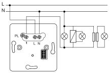
Insert with mechanical push-button via PlusLink
