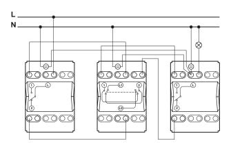
2 two-way switches + 1 intermediate switch with indicator lamps
