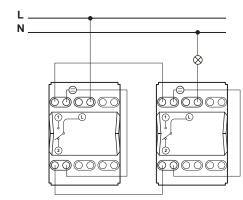
One-way switch with locator lamp
