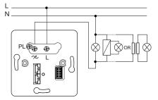
Insert with a mechanical push-button via PlusLink
