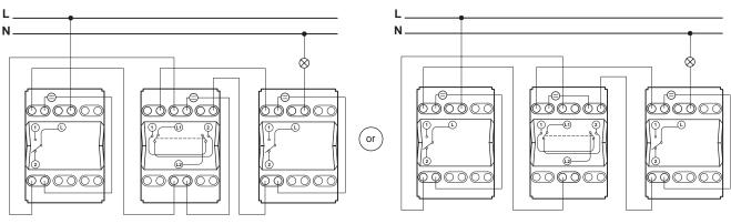
2 two-way switches + 1 intermediate switch with locator lamps
