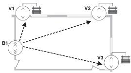
The 3 combined modules for roller blinds V1, V2, V3, (receivers) are installed in place of the
