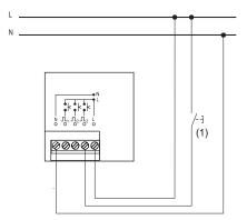
(1) Use of a maximum of 10 push-buttoms without indicator lamp connected in parallel or 3 push-buttoms with indicator lamp connected in parallel.
