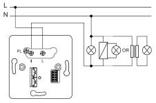
Insert with mechanical pushbutton via PlusLink
