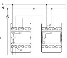
2 two-way switches with indicator lamps
