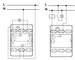
Double pole switch with locator lamp
