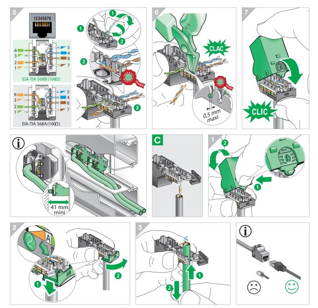
Installation Example of shielded data socket installation (cat 5e)
